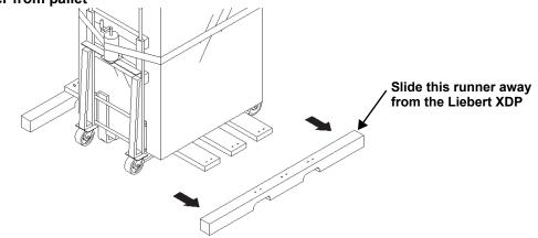
Using the pallet jacks, raise the secured unit to the highest point that the piano jacks will allow. Once the unit has been raised, slide the remainder of the pallet from under the Liebert XDP (see Figure 7). Lower the Liebert XDP so that its base is approximately 1" (25.4mm) off the ground.
